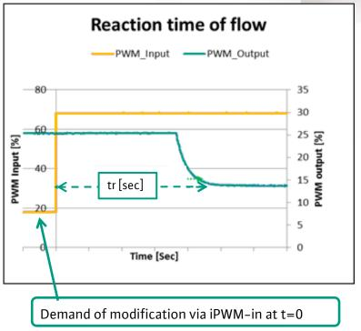
If the controller adjusts iPWM-in with a higher frequency than the "reaction time", the flow data sent by iPWM-out may not be updated. However the rotation speed will change according to the demand.
